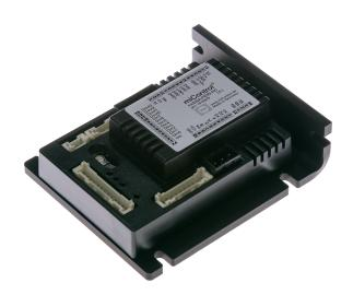
The mcDSA-FE55 series combines modern control technologies with an optimized control structure. By implementing vector commutation, the new controllers enable smooth and quiet running even at low speeds, reduced noise emissions and outstanding performance, for example with external rotor motors.
